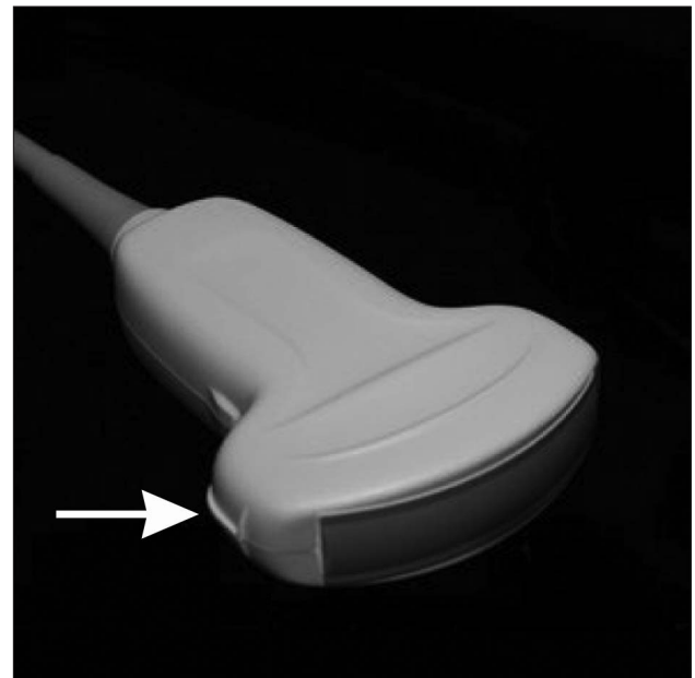
Fig. 1. Low-frequency (2–5 MHz) curvilinear probe. The probe marker (arrow) should always be pointed toward the patient's right side.
